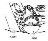
Tilt cover to back. Press cover firmly until side tabs snap into place. Replace cover screws, light bulb and light cover.
