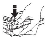
4) Line up front cover and base. Rest cover on front edge of base as shown.
