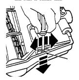
Tirm brush over. To remove cover, insert screwdriver at cover tabs on both sides and twist to release tabs.
