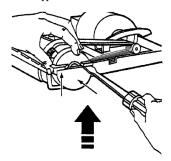
6) Remove broken or worn belt.
