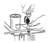
Turn brush over. To remove cover, insert screwdriver at cover tabs on both sides and twist to release tabs.
