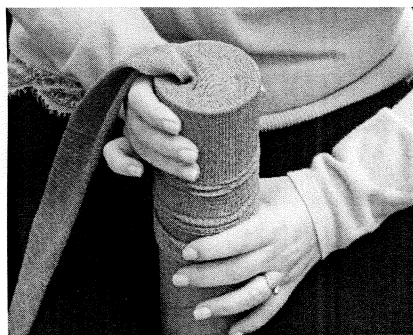
2. Push in downward motion until the entire VacSoc® is on tube.
